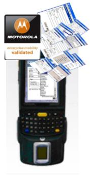
The system is an integrated mobile computer, a Motorola MC75, fingerprint scanner, digital camera, 2D barcode reader, and support of wireless communications. In addition, PrintSearch Mobile provides inthe-field mobile positive identification, for electronic ticket writing, pre-booking, and book and release, with notice to appear documents.
